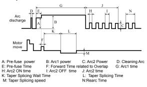
Diagram of ARC discharge condition
